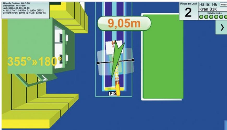
Figure 4. The cabin monitor shows the coil from a perpendicular perspective
