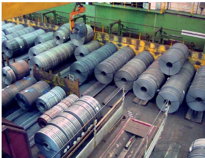
Figure 1. Storage area for the coils coming from the two pickling lines
