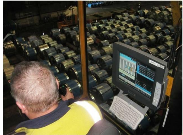
Picture 1 - WMS terminal in crane cabin
